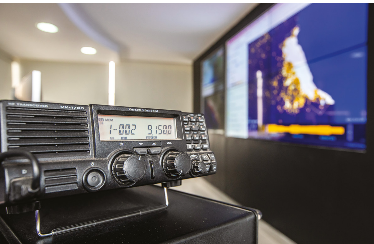
Inside a fisheries monitoring and control center, a high-frequency marine radio sits ready for direct communication with vessels. In the background, the Global Fishing Watch map provides a clear picture of coastal vessel presence using VMS data. © Global Fishing Watch
