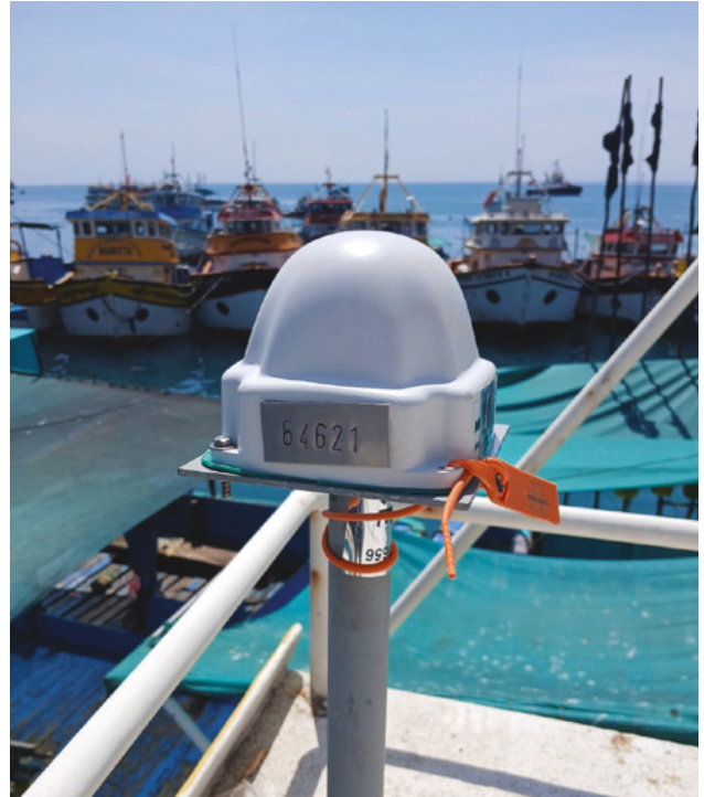
A type B VMS satellite terminal mounted on a Peruvian vessel. The unit is secured to the mounting bracket with an orange tamper-evident seal to ensure data integrity and compliance. © SISESAT-PRODUCE-PERU
