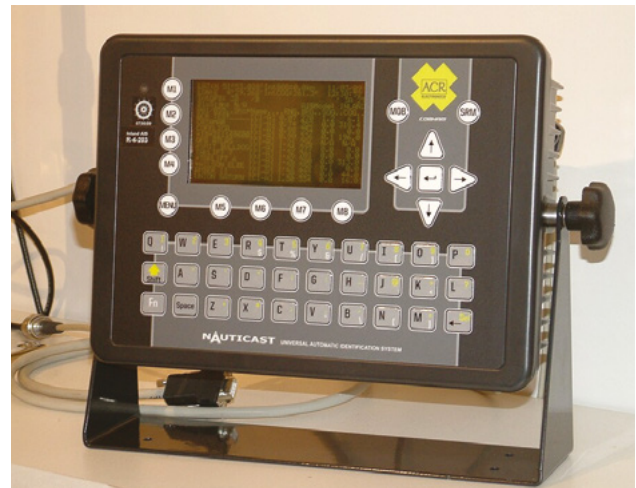
An onboard AIS transponder features a built-in display screen and keyboard for manual data entry. © Wikimedia commons
